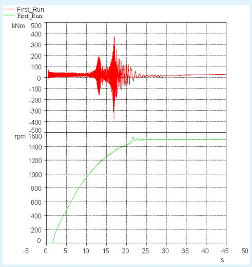
Torque curve and speed during start-up of a turbo compressor
